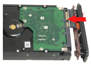
**Step 3** With the hard drive label facing up, attach the guides to both sides of the hard drive.
